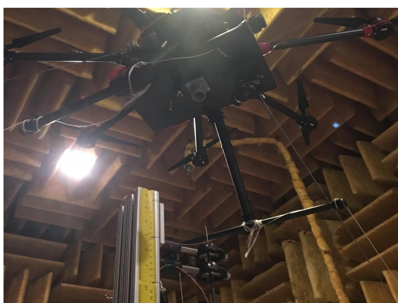
Figure 3: Traversing hotwire positioned beneath S1000 to acquire profile of freestream velocity of the crossflow that is interacting with the drone's downwash.
